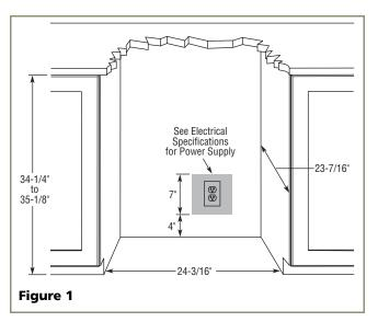
Follow the cut-out drawing in **Figure 1**. The 24-3/16" width allows 1/4" for ease in installation and removal of the unit. 24" is the counter depth in most installations. The unit is 23-7/16" deep including the door and *not* the handle on Stainless models and 23-7/16" deep including the handle on Black and White models (see **Figure 2**).
